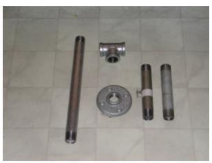
was a foot long. Then, a t-joint plus two more flanges each about 6 inches long. Finally, I found a footer, to make the base of the core blaster.
